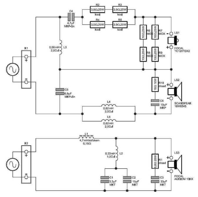
L1 = 4.7 mH transformer inductor, R = 0.14 ohms (tolerance 5% - matched pair 1%)
